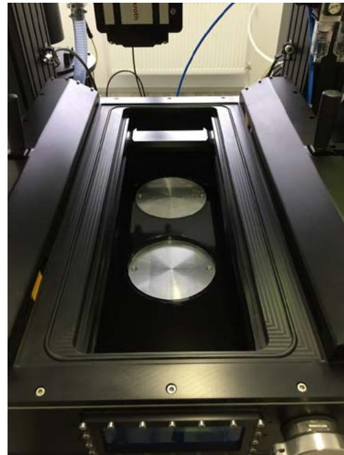
Laboratory dedicated 3D printer of metallic materials with selective laser melting (SLM) with possibility of substrate preheating.
