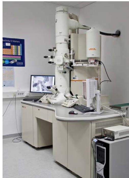
State-of-the-art electron microscopes (SEM, TEM), which provide insight into the microstructure of metallic materials all the way to the atomic level.
