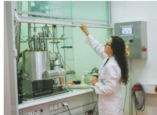
Laboratory mixing reactor for polymer synthesis
